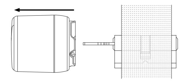
Heat the adapter with a hair dryer for 10-15 minutes and try to remove it with a flathead screwdriver. If unsuccessful, repeat the process until the adapter is removed.
