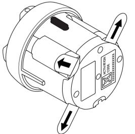
After removing the third protective tab, check for a light signal (LED). The RED-GREEN-BLUE-WHITE sequence confirms that your Tedee GO is ready.
