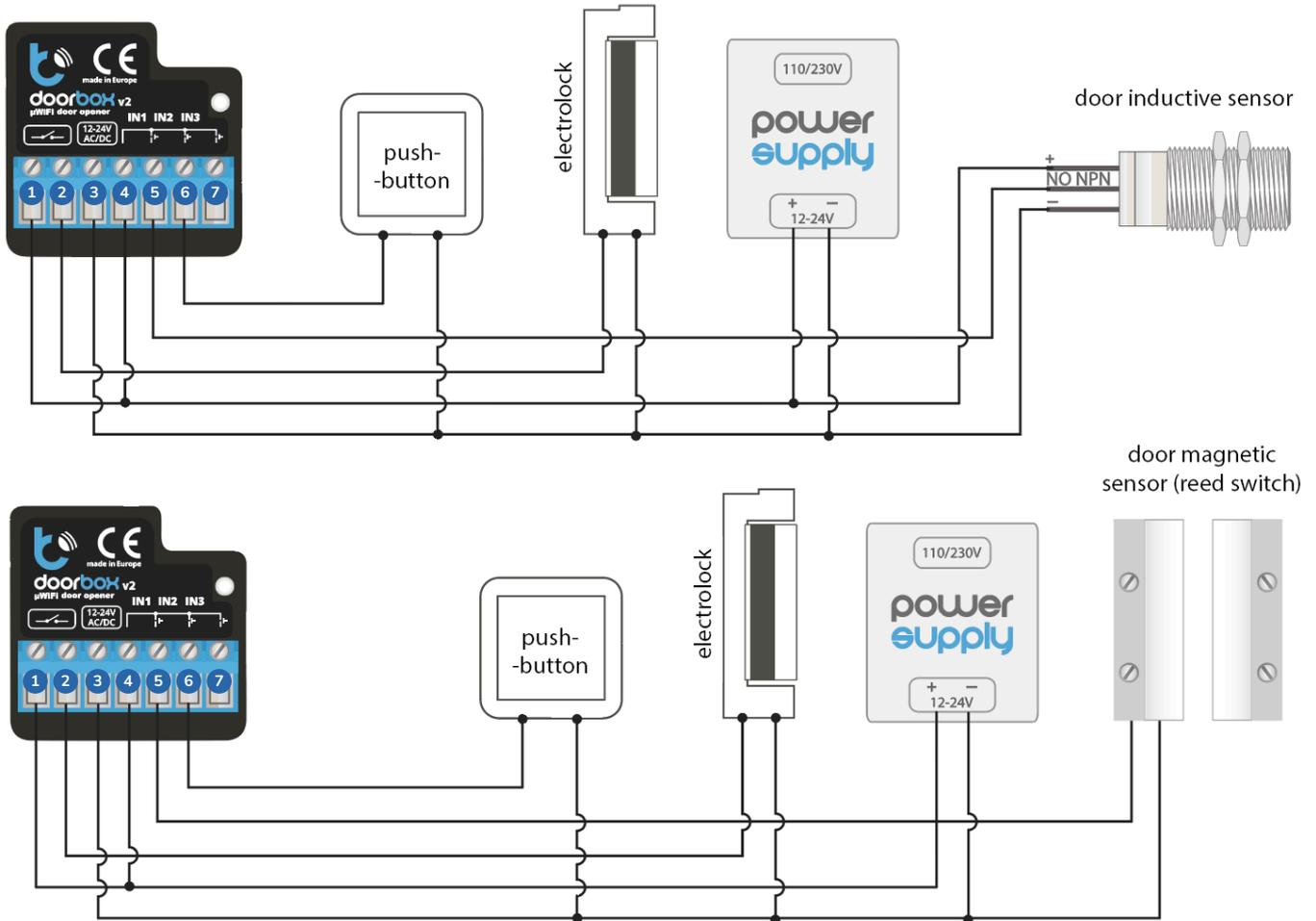
Start by connecting the +12V or +24V power to the [12-24 AC/DC] inputs (3) & (4) as shown on the drawings above.
