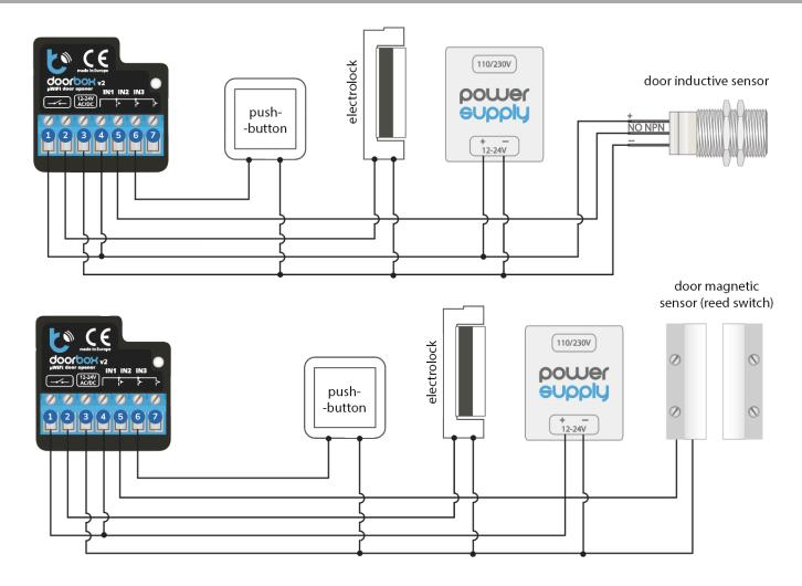
Start by connecting the +12V or +24V power to the [12-24 AC/DC] inputs (3) & (4) as shown on the drawings above.
